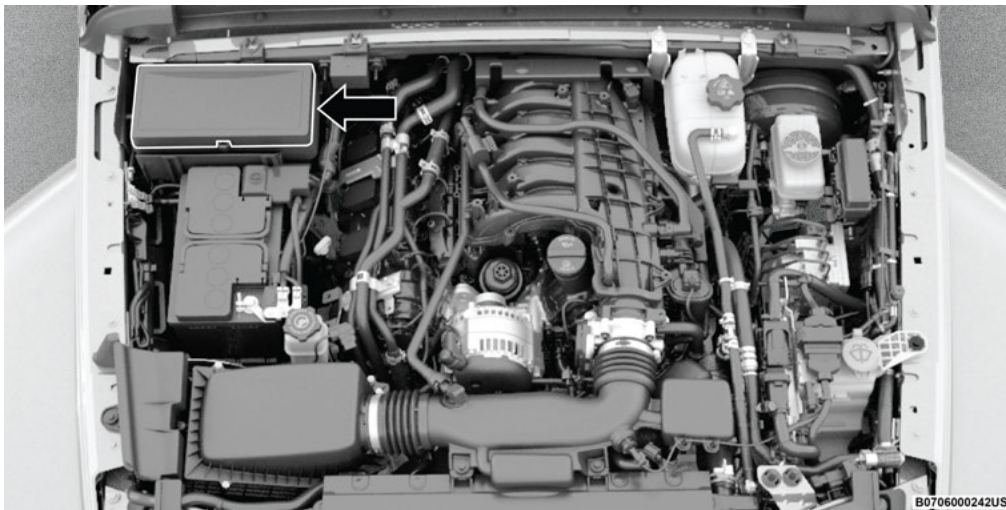
Power Distribution Center Location - Gasoline Engine
