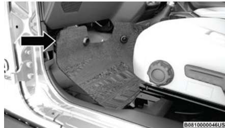
Front Carpet Pulled Away
