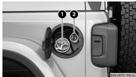
Fuel and Diesel Exhaust Fluid Fill Location
