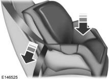
8. Remove remaining slack from the belt. Force the seat down with extra weight, for example, by pressing down or kneeling on the child restraint while pulling down on the lap belt in order to force slack from the belt. This is
