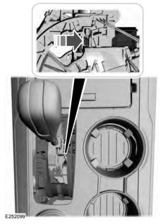
**Note:** Do not press the upper metal lever, damage to vehicle may occur.
