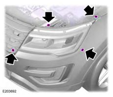
To gain access to the headlamp securing bolts and to remove the headlamp assembly, you must first remove the front fascia and front bumper assemblies. We recommend you see an authorized dealer.
