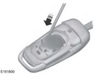
**Note:** Do not touch the battery contacts or the printed circuit board with the screwdriver.
