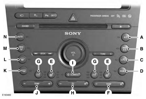
A **A/C:** Press to switch the air conditioning on or off. Use A/C with recirculated air to improve cooling performance and efficiency.
