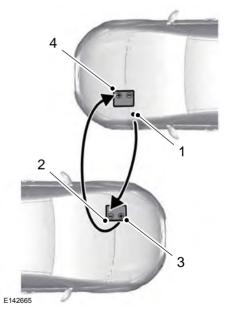
1. Remove the negative (-) jumper cable from the disabled vehicle.
