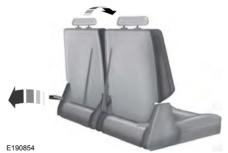
3. From the rear of the vehicle, fold the seatback by pulling and holding the red strap while pushing the seatback forward. Release the strap once the seatback starts rotating forward.
