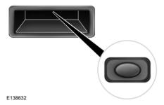
Press the button located in the top of the liftgate pull cup handle to unlatch the liftgate, and then pull on the outside handle.
