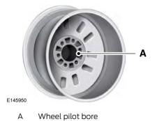
Inspect the wheel pilot bore and mounting surface prior to installation. Remove any visible corrosion or loose particles.
