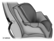
2. After positioning the child safety seat in the proper seating position, grasp the shoulder belt and lap belt together behind the belt tongue.
