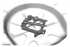
With the road wheel in the vertical position in the spare tire tub, the jack assembly will not fit in its standard position. Secure the jack in the alternate position by inserting the wing bolt through the jack as shown.
