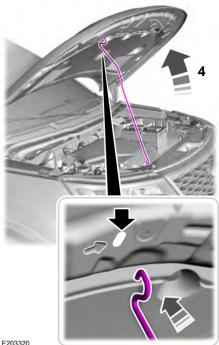
4. Open the hood. Support the hood with the strut.
