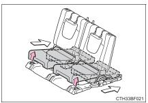
3 Pull the lever to unlock the seatback and then fold the seatback down.
