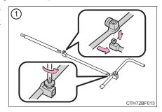
② Assemble the jack handle extension bars and tighten the bolt.
