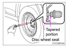
When replacing an aluminum wheel with an aluminum wheel, tighten the wheel nuts until the washers comes into contact with the disc wheel.
