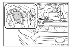
5 Add engine coolant if necessary. (→P. 422)
