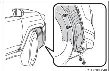
3 Partly remove the fender liner.
