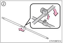
3 Assemble the jack handle and the jack handle extension bar and tighten the screw.
