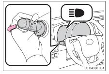
2 Press the Automatic High Beam switch.
