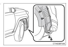
3 Partly remove the fender liner.
