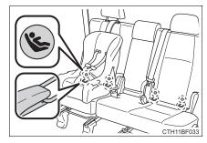
Seat belts equipped with a child restraint locking mechanism (ALR/ELR belts except driver's seat belt) (→P. 33)
