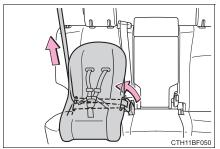
5 If the child restraint has a top tether strap, the top tether strap should be latched onto the top tether strap anchor. (→P. 68)
