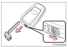
After using the mechanical key, store it in the electronic key. Carry the mechanical key together with the electronic key. If the electronic key battery is depleted or the entry function does not operate properly, you will need the mechanical key.  $(\rightarrow P. 520)$
