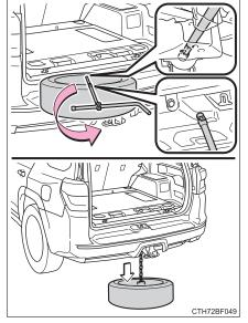
3 Pull out the spare tire and remove the holding bracket.
