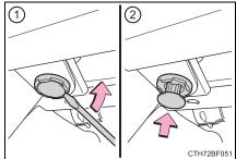
Securely attach cables or chains to the towing hook.
