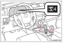
The initial shift range in S mode is set automatically to "4" according to vehicle speed. However, the initial shift range may be set to "3" if Al-SHIFT has operated while the shift lever was in the D position. (→P. 218)
