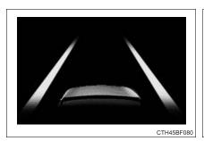
Indicates that the system is recognizing white (yellow) lines. When the vehicle departs from its lane, the white line displayed on the side the vehicle departs from flashes yellow.
