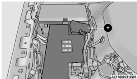
Positive (+) Battery Post
