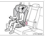
Check that the shoulder belt is correctly positioned over the child's shoulder and that the lap belt is as low as possible. ( $\rightarrow$ P. 30)
