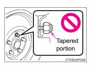
Never use oil or grease on the wheel bolts or wheel nuts. Oil and grease may cause the wheel nuts to be excessively tightened, leading to bolt or disc wheel damage. In addition, the oil or grease can cause the wheel nuts to loosen and the wheel may fall off, causing an accident and resulting in death or serious injury. Remove any oil or
