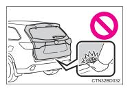
Use caution when using the back door closer as it still operates when the power back door system is canceled.
