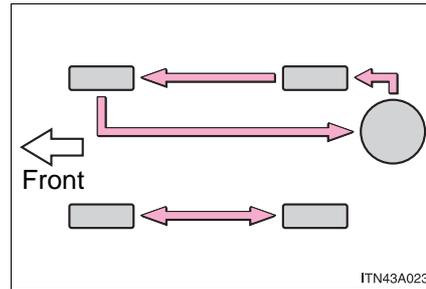
Do not fail to initialize the tire pressure warning system after tire rotation.
