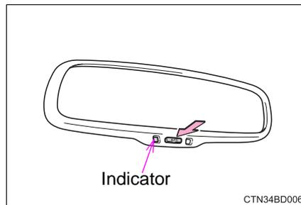
When the automatic anti-glare function is in ON mode, the indicator illuminates.
