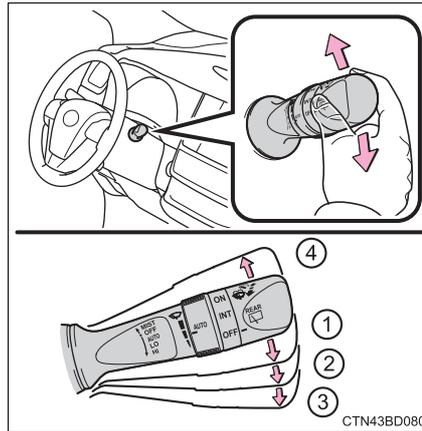
When AUTO mode is selected, the sensor sensitivity can be adjusted by turning the switch ring.
