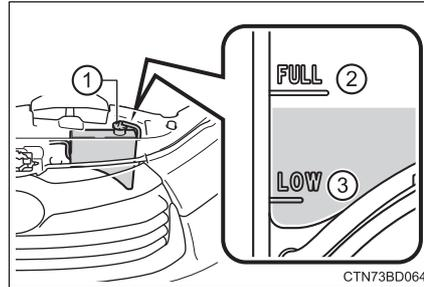
► Power control unit coolant reservoir
