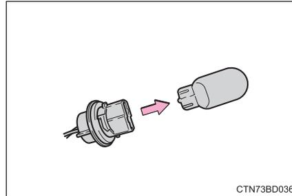
**5** When installing the light bulb, install by conducting **4**, **3** and **2** with the directions reversed.
