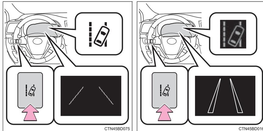
Press the LDA switch to activate the system.
