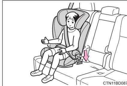
Check that the shoulder belt is correctly positioned over the child's shoulder and that the lap belt is as low as possible. (→P. 32)
